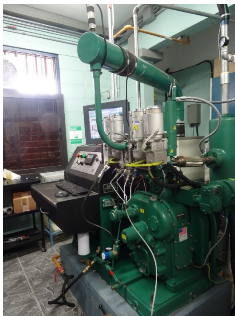
CFR Engine ASTM D2700-22 test
